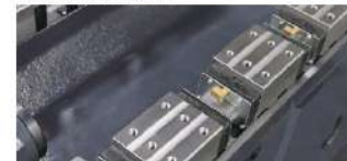
X/Z axis roller linear guideway with 3 sliders
