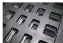
Base, worktable, and gantry beam all adopt a box-shaped double-layer rib structure.
