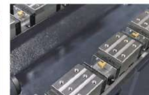
X-axis and Z-axis use the linear guideway with 3 sliders Ensure the large load capacity of worktable and cutting rigidity of the Z-axis.
