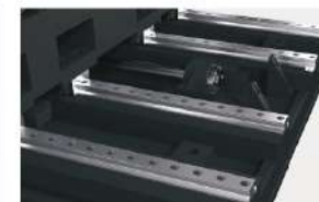
Y-axis has 4 linear guideway X-axis support is more stable, it can improve processing stability.
