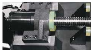
Three-axis hollow oil-cooled ballscrew
