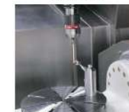
Workpiece's online measurement and rotary table center automatic calibration system
