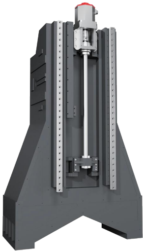
Larger and wider span herringbone design The interior adopts dense and thickened rib arrangement, compared with ordinary columns, the body's rigidity, torsion resistance and bending resistance are enhanced. The contact area with the base is increased, the processing more stable accordingly.
