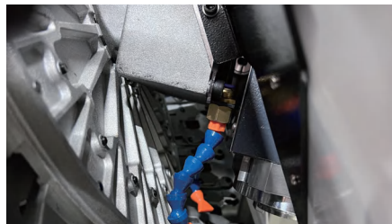
Tool holder cleaning function before tool exchange
