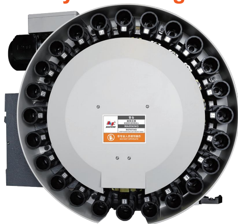
ATC adopts advanced tool clamping technology Tool change time 2.3 s (T to T)
