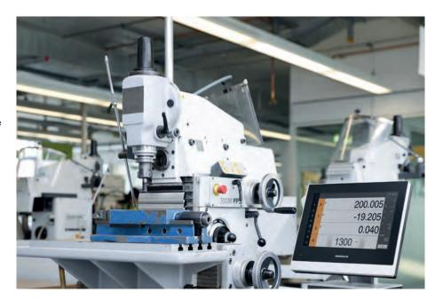
Distance-to-go mode comes to your aid during positioning tasks. With it, you can easily and reliably arrive at the next position by simply moving the axes until the display reads zero. This feature is particularly useful during the execution of programs.
