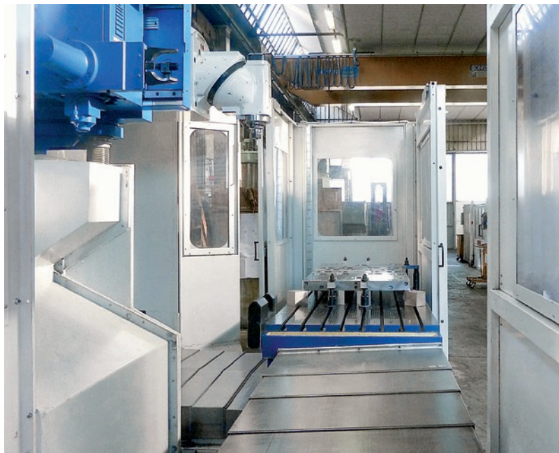
"T"-morphology: transversal moving column with no ram
