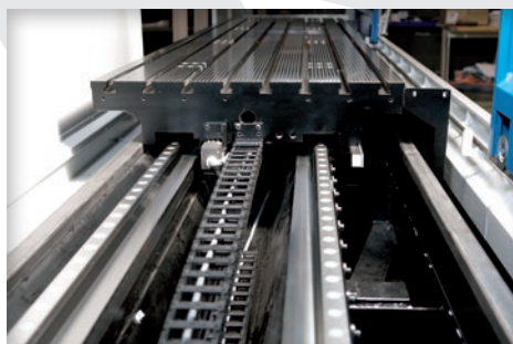
X axis with double motor/ pinion on precision rack with electronic backlash recovery
