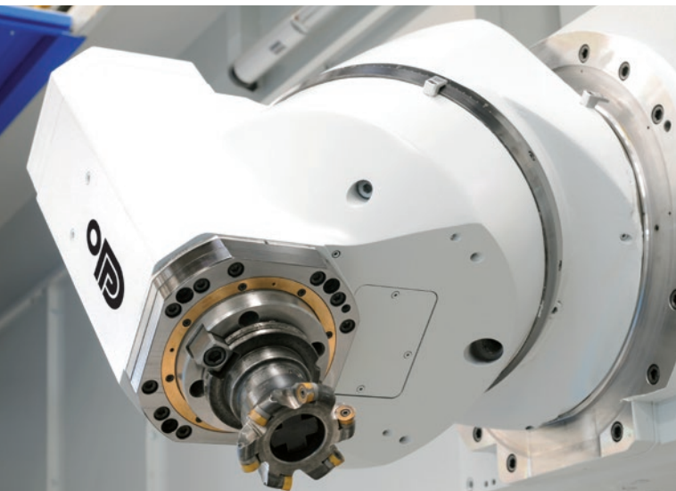
High-stiffness universal milling head (power up to 33 kW)
