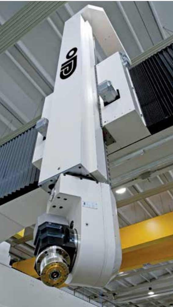
Crossbeam structure optimised for ensuring the necessary accuracy and stiffness even with the completely extended ram
