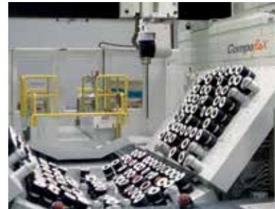
Speeder can integrate CompoX, the universal flexible tooling system developed by Jobs that allows the reference and clamping of composite parts
