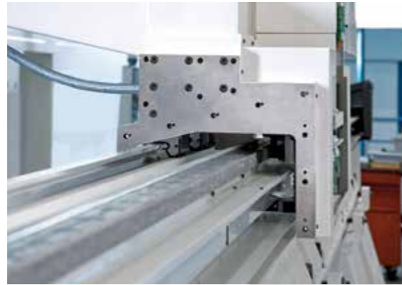
Longitudinal axis frame (X axis) optimised for the best compromise solution between dynamics, accuracy and axis stiffness
