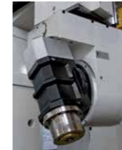
T2D-04 head with HSK-A-63 spindle 24000 rpm and power up to 22 kW
