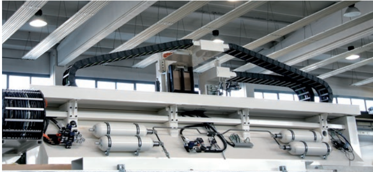
Very efficient hydro-pneumatic counterweight system, for balancing masses of Z-axis group, composed of a direct dual cylinder
