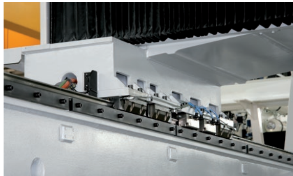
Large-size longitudinal structure (X axis) on which wide-section guides with preloaded rollers are fixed and installed on columns
