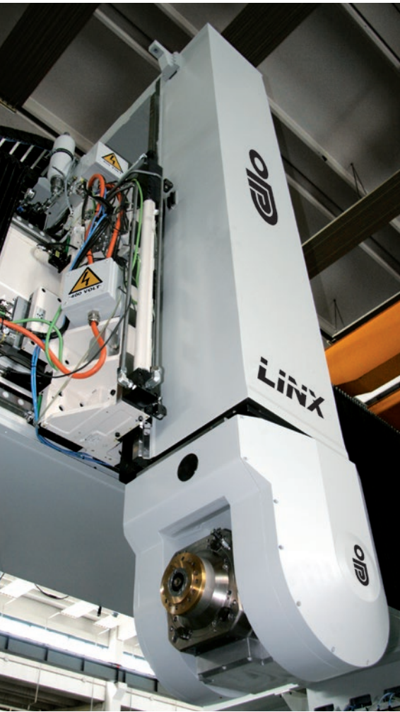
Large-size longitudinal structure (X axis) on which wide-section guides with preloaded rollers are fixed and installed on columns
