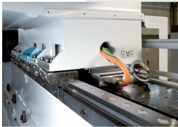
Vertical axis frame (Z axis) composed of a ram sliding within the saddle on wide-section guides with preloaded rollers
