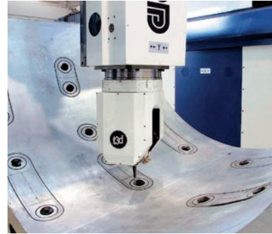
T3D Aero-configuration head for high-power machining in aerospace industry
