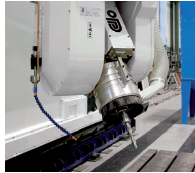
Bipolar T2D head for car design & prototyping applications
