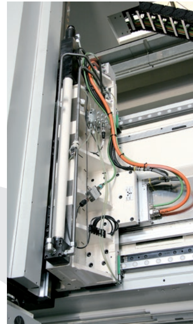
Transversal axis frame (Y axis) composed of a duly optimized crossbeam with wide-section guides and preloaded rollers for saddle movement
