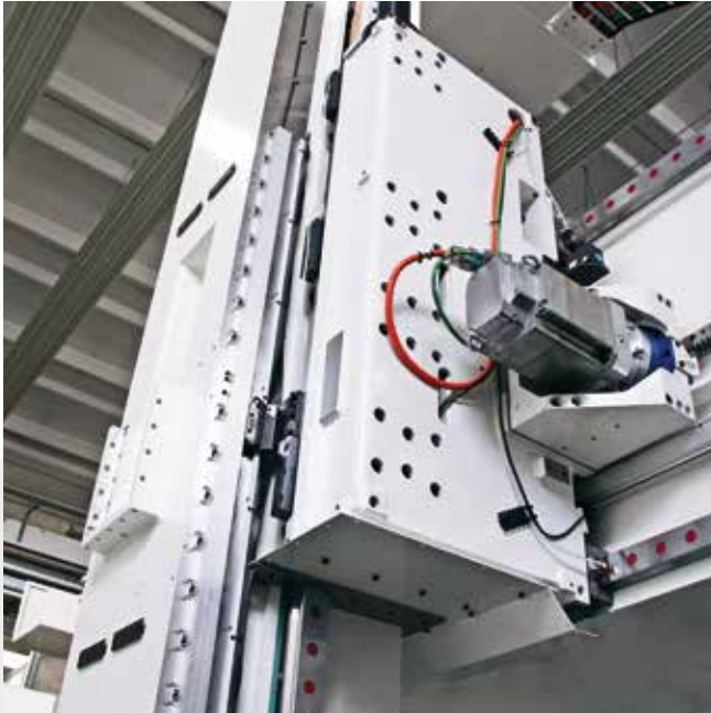
Transversal axis frame (Y axis) composed of an electrowelded metal structural work crossbeam with two guides with preloaded rollers for Y-axis saddle movement
