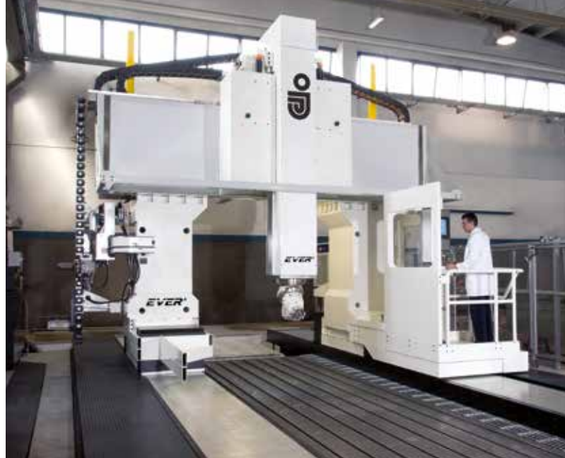
MT frame: crossbeam structure with multi-triangle section conceived for the highest torsional and bending stiffness and for high dynamic efficiency
