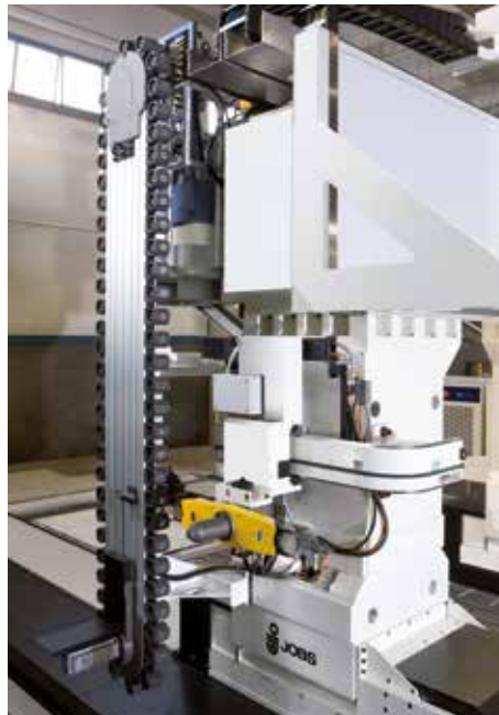
Chain-type tool magazine with 40/60 positions ISO50/HSK-A-100
