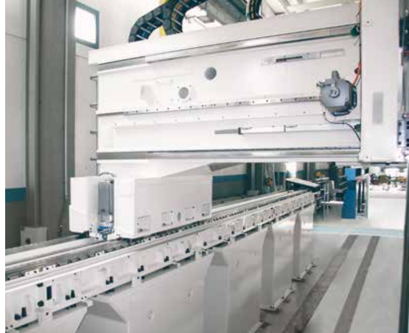
MT frame: longitudinal axis frame (X axis) with multi-triangle section conceived for the highest torsional and bending stiffness and for high dynamic efficiency
